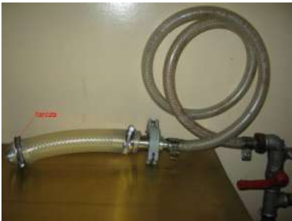
Fig. 4. Water tightness check.
