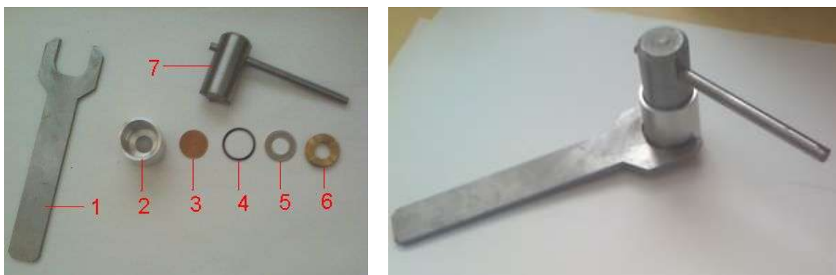
Fig. 2. The modified target assembly for activation of zinc at the PETtrace cyclotron.
