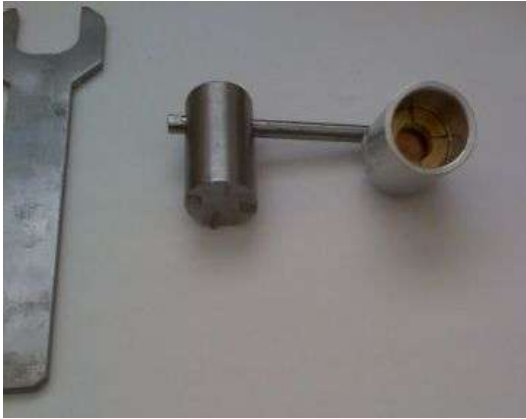
Fig. 3. The assembled target shuttle and its two dedicated wrenches; rear (left) and front (right) views.
