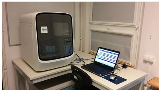
Figure 8. The RT-PCR system for real-time testing of DNA sequence. Research involved: gene expression studies, single nucleotide polymorphism (SNP) searching, dysfunctional copy number of the gene (CNVs), \mu RNA profiles, detection of pathogens.
