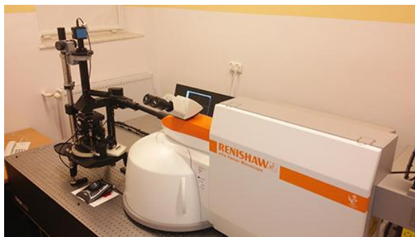
Figure 2. The integrated Raman-AFM system capable of performing Raman microscopy, atomic force microscopy (AFM) and Raman nanospectroscopy enhanced on the AFM tip (TERS).
