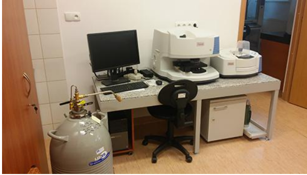
Figure 5. Independent fast imaging IR microscope (Nicolet IN10 MX) – for spectral imaging and spot measurements, equipped with three detectors and motorized microscope table. Capable of recording the spectrum in both transmission and reflection modes, as well as of taking classical microscope images of the sample.
