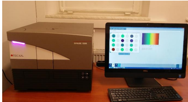
Figure 6. UV-VIS Spectrometer - plate reader – (spectrophotometer Spark M10), allowing the use of multiple absorption, fluorescence and luminescence markers.
