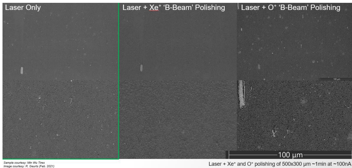
Figure 1. Tire polymer cut face from laser only, laser+Xe ion polishing and Laser+O ion polishing, respectively.
