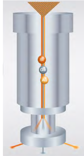
Left: General VELION setup with vertical FIB column on Laser Interferometer Stage and SEM Right: Multi ion species FIB from Liquid Metal Alloy Ion Sources.
