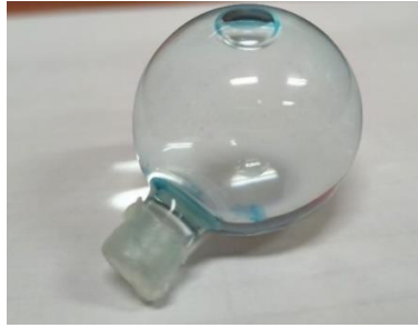
Figure 14 Spherical \text{CuSO}_4 phantom for trajectory measurement
