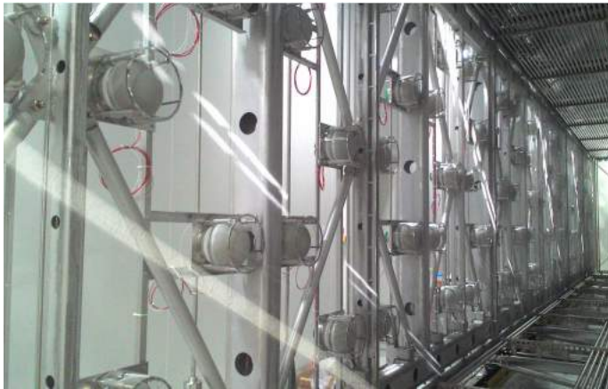
Figure 6.2: PMTs installed on the ICARUS detector wall according to the schematic shown in Figure 6.1. Figure from [2].
