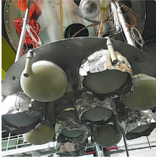
Figure 8.2: The 10 PMTs that formed the light detection system for the LAr test facility at CERN. The number of PMTs with TPB coating has been reduced to 6 replacing 4 PMTs with PMTs without TPB coating. Aluminium screens have been installed to isolate the PMTs with the TPB deposition to limit the optical cross-talk caused by them. Figure from [8].
