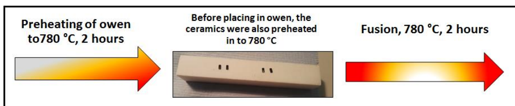
Fig. 4.5. Scheme of the process of fusion of microsphere with the cantilever in the oven.
