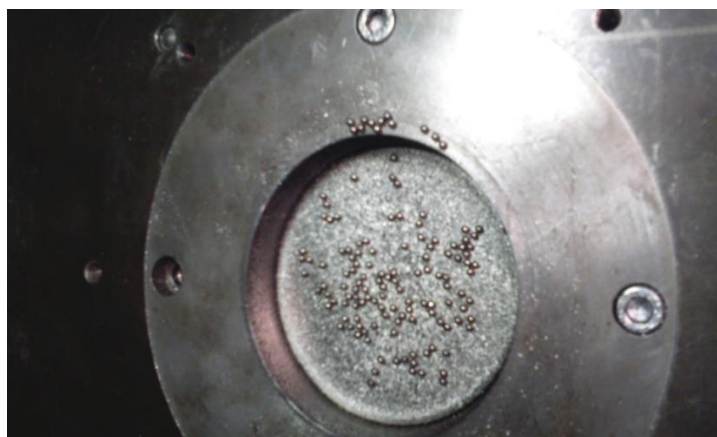
Figure 7.1 Mg specimen after the SMAT.
