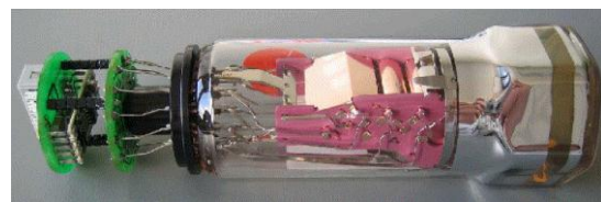
Figure 3.8: The photomultiplier tube (Photonis XP3062), which is used in the cameras of FD telescopes at the Pierre Auger Observatory.
