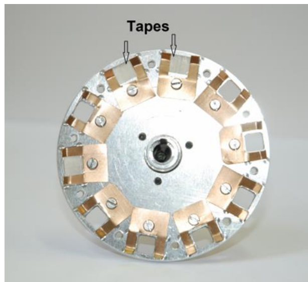
Fig.5 Two samples of 2G HTS mounted on the Carousel [13].
