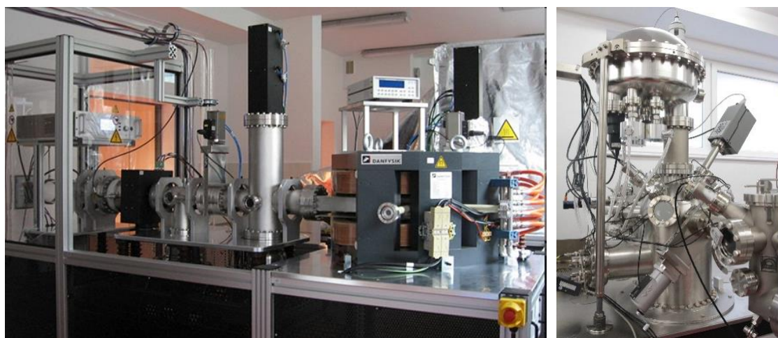
Fig.10 The UHV accelerator system at the University of Szczecin. Left: ECR ion source and analyzing magnet. Right: Target chamber
