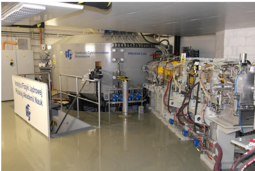
Fig.5 The Proteus C-235 isochronous cyclotron at the Cyclotron Centre Bronowice, IFJ PAN. (copyright: K. Gugula)
