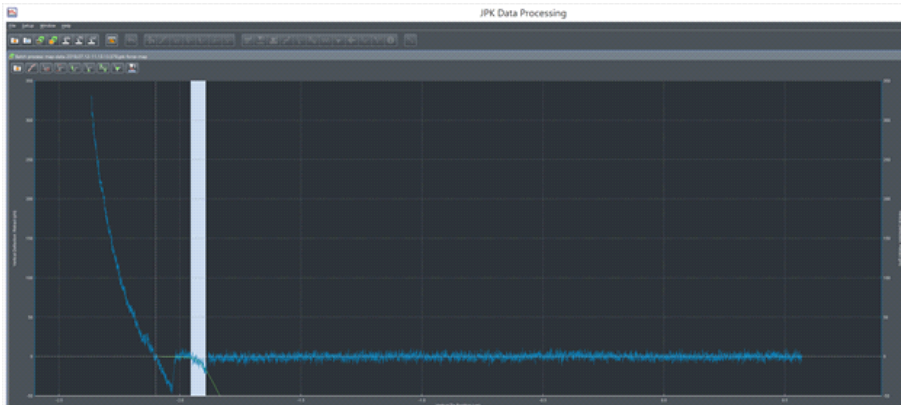
Figure 9: The example of a retract force curve registered during measurement of HCV29 collected within the DFS experiment using Nanowizard 4 AFM head and MabSDC-1 functionalized probe. The part of the curve that corresponds to specific unbinding event is marked in white (approximately 1.9 \mu\text{m} vertical tip position). The unbinding event around 2.1 \mu\text{m} vertical tip position denotes un-specific adhesion bond break. The green curve is fitted according to Extensible Worm-Like-Chain model further described in the chapter 3.5.
