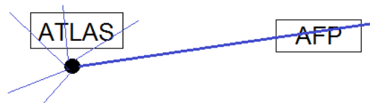
Figure 7.1: Scheme of the signal process. The solid black dot represents the reconstructed vertex and the thick blue line a track reconstructed in the AFP.
