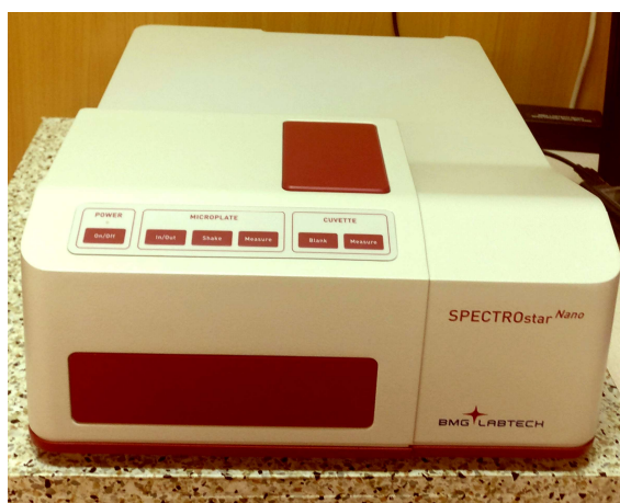
Figure 13. SPECTROstar Nano - spectrophotometer for the ELISA method working at the IFJ PAN.
