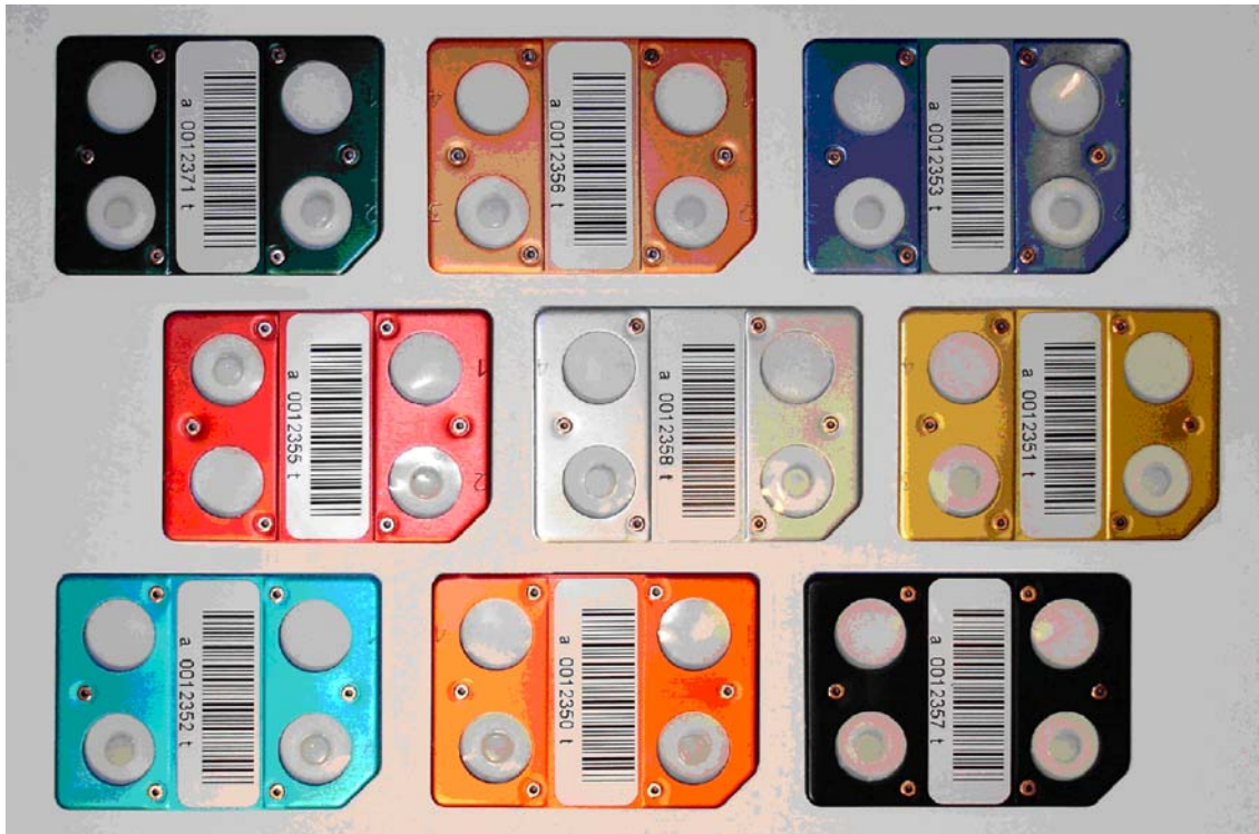
Fig. 1. TLD European Card (TLD-EC) with 2 MCP-7 detectors in positions 2 and 3
