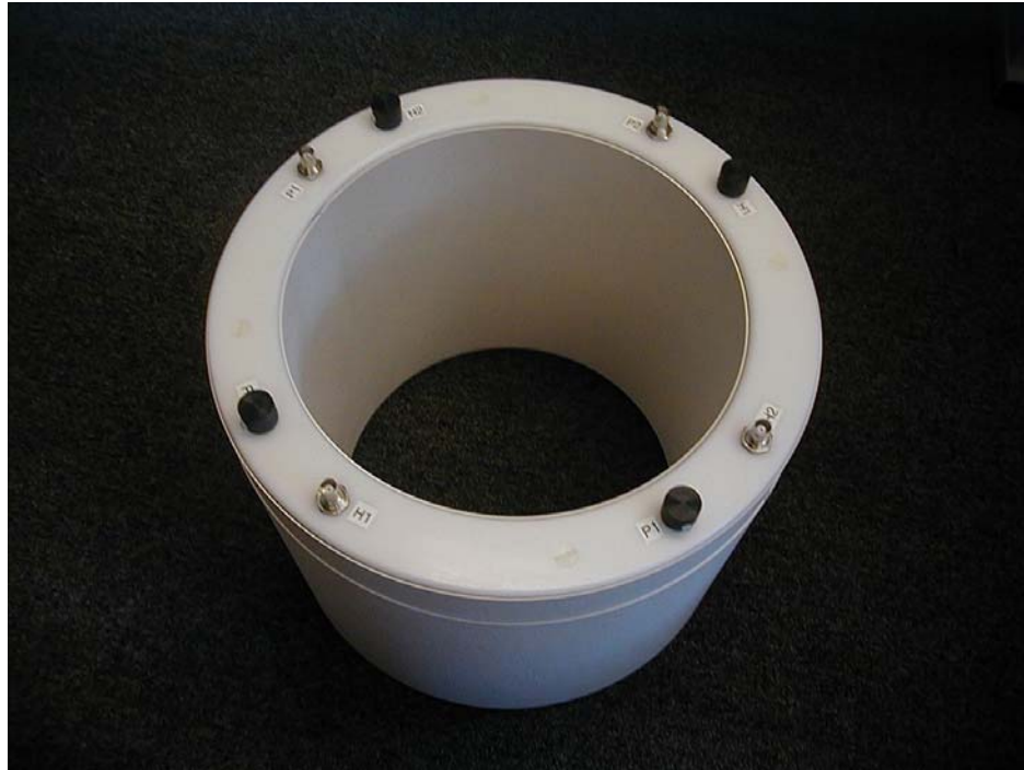
FIG. 8.1 - Example of a standard RF quadrature birdcage for a human head (such a coil cannot accommodate skull clamp)
