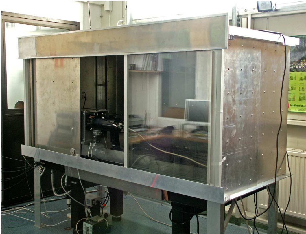
Fig. 2. Optical table and radiation shielding of the X-ray microprobe
