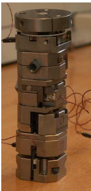
Fig. 5. Goniometer used in the CMT experiments
