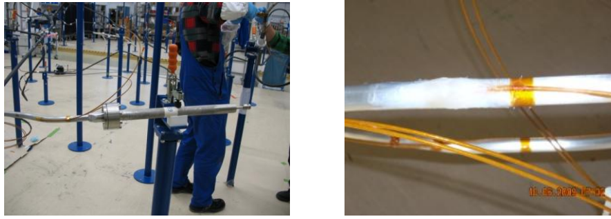
Fig.11 One end of a bus bar prepared for vacuum test after welding of T&C piece (left), two additional QD wires bonded to the Al jacket (right)
