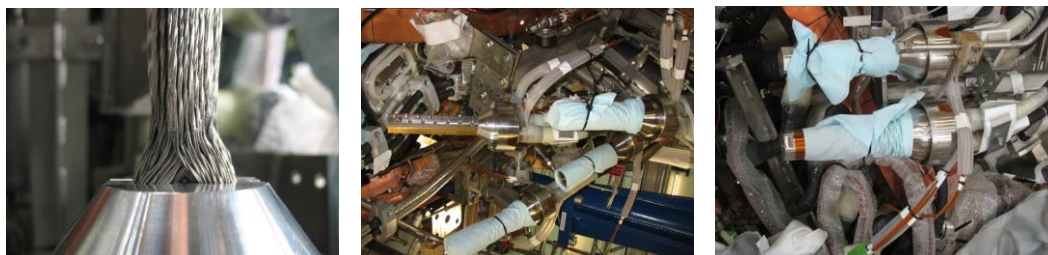
Fig.16 Various phases of joint assembly; transition region shaped with special tools (left), superconducting triplets squeezed with bi-metallic clamp (centre), welded joint ready for insulation (right)
