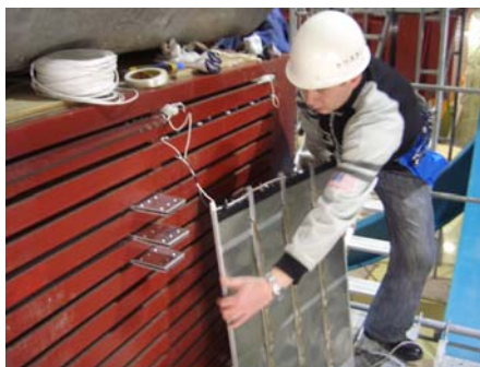
Fig. 37 One horizontal module with read out cables before the installation in the magnet slit (left); the module in the magnet slit (right)
