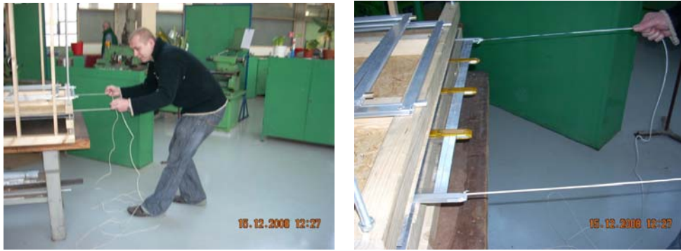
Fig.19 Extraction of the modules from the magnet slits using ropes
