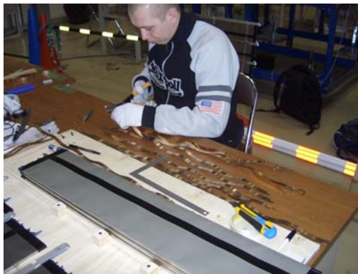
Fig.30 Adjustment of the springs length
