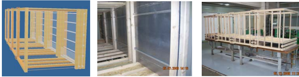
Fig.4 Mockup of four magnet towers: AutoCAD drawing (left), set vertically (centre) and horizontally (right)
