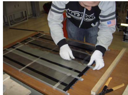
Fig.31 Installation of the springs
