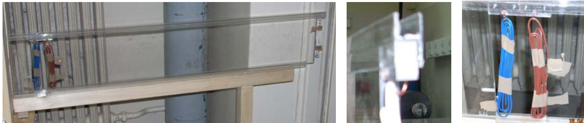
Fig.7 Single dummy counter with necessary accessories (H-rails, cables) inserted into the magnet mockup
