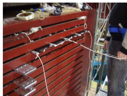
Fig. 37 One horizontal module with read out cables before the installation in the magnet slit (left); the module in the magnet slit (right)
