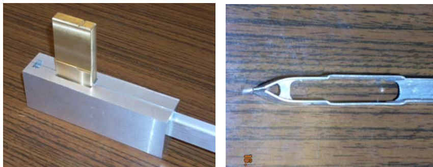
Fig.23 The tool to widen H-profiles (left); a widened H-profile (right)
