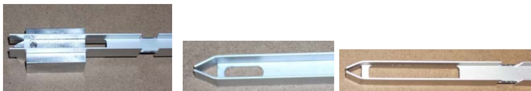
Fig.22 The tool to taper ends (left) of C-profiles (centre) and H-profiles (right)
