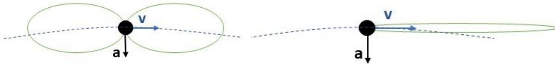
Figure 26 Schemes of the angular distribution of emitted radiation by the accelerated electron
