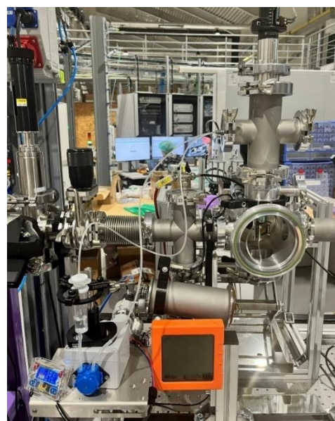
Figure 85 Liquid delivery setup, which was mounted on the ASTRA beamline of SOLARIS
