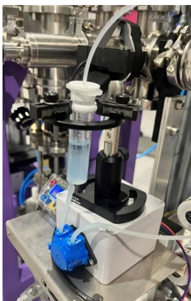
Figure 84 Part of the liquid delivery setup, with presented container from the part of syringe, and little peristaltic pump controlled by the microcontroller
