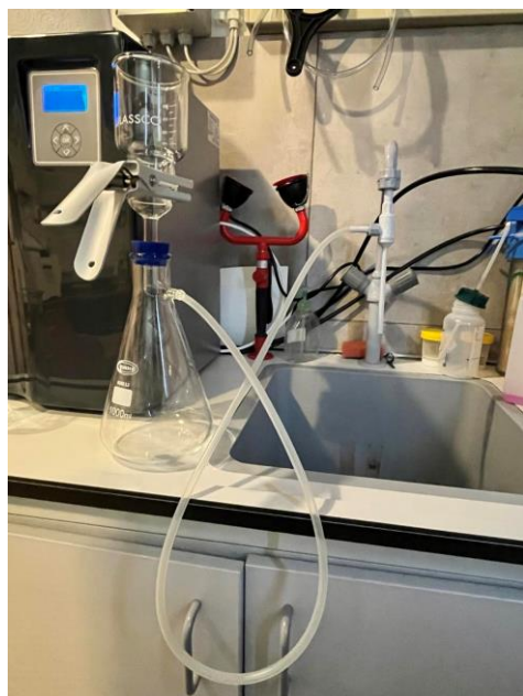
Figure 11 Filtration setup connected to the water pump
