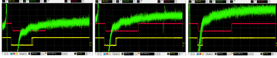
Figure 6.9 Constant input signal amplitude equivalent to lower energy component of ^{207}\text{Bi} spectrum (green). Only the lowest part of the signal is visible. Controlled variation of baseline position of input analog signal (green) with a step of 2 mV is done. Resulting drastic change of width of respective converted output pulse (yellow) is visible.
