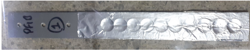
Figure 3.16 The gold foil embedded within the aluminum frame forming 10 circular areas. The gold foil is additionally protected by a layer of Al film. The circular spots of gold foil are used for the beam profile measurement via the neutron induced activation with the reaction: n + {}^{197}\text{Au} \rightarrow {}^{198}\text{Au} \rightarrow \gamma, \beta \rightarrow {}^{198}\text{Hg}
