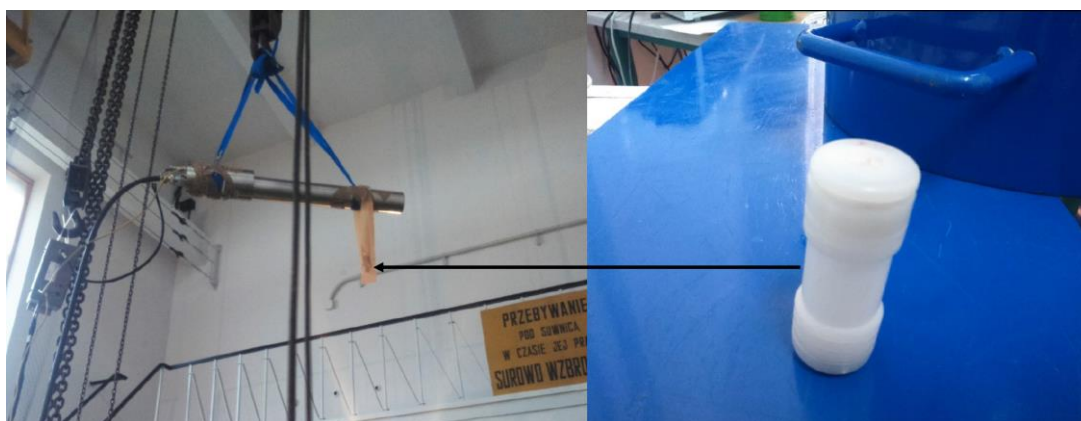
Figure 10.37. The location of the Sodern Genie 16C during the experiment (left) and capsule with dosimetry foils (right) [Las2017].
