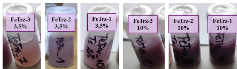
Figure 5.3.1 Photographs of electrospinning polymer suspensions of FeTrz-1 , -2 , and -3 .
