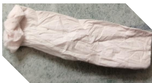
Figure 5.3.2 The photography of electrospun composite of the FeTrz-2/PVP-20% fibres.
