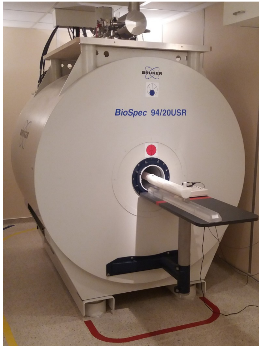
Figure 36: Bruker BioSpec Avance III MRI 9.4 T.
