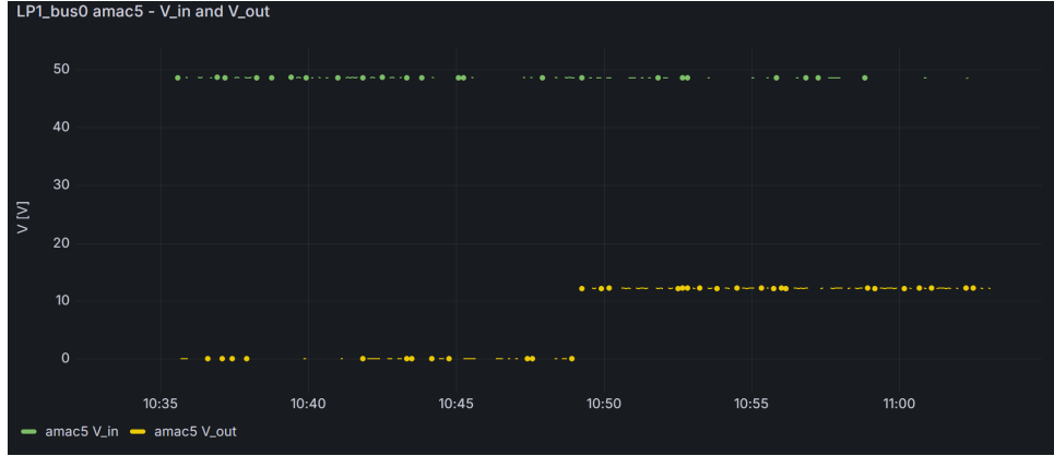
Figure 35: Grafana panel providing monitoring of the input/output voltage for a specific AMACstar chip before and after enabling the DC/DC converter.
