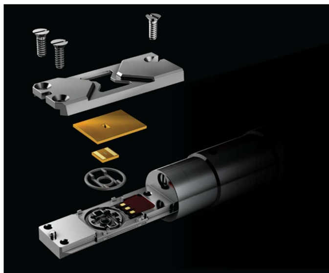
Figure 6 Poseidon Select system for liquid cells consisting of: bottom plate of the holder, seal (the O-ring), bottom chip of the liquid cell (with 2 yellow spacers), top chip, and top plate of the holder. On the bottom plate of the holder 3 golden contact electrodes for electrochemical experiments are located. Reproduced from Tarnawski and Parlińska-Wojtan, 2024. Copyright 2023 Protochips.
