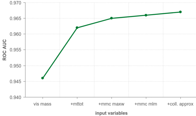
Figure 8.5: ROC AUC values of BDTs trained on Z/\gamma^* \rightarrow \tau^+\tau^- background and 200 GeV ggH/A+bbH/A signal in the b -veto category, using different mass variables.
