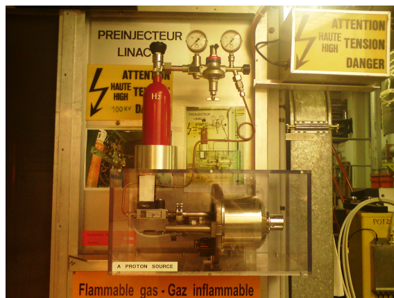
Figure 4.2: LHC protons originate from a small hydrogen bottle, pictured here with the duoplasmatron. [140]
