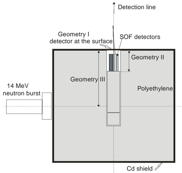
Fig 2. Three types of geometry in the experiments with the SOF detectors.
