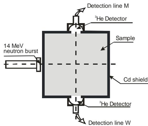
Fig. 1. Experimental set-up with  $^3\text{He}$  detectors at the fast neutron generator.
