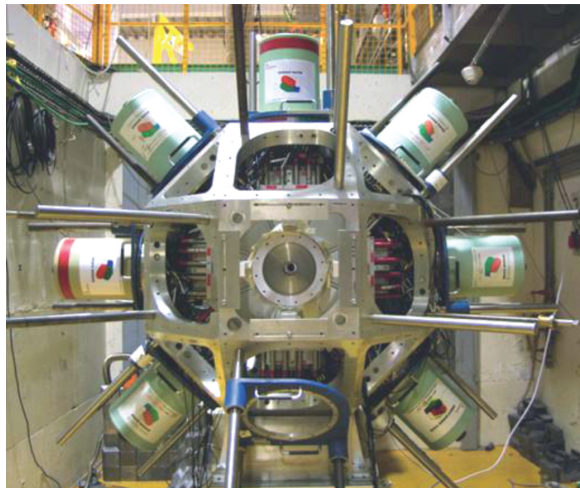
Figure 3.8. A picture of the real setup of the EXOGAM ring.
