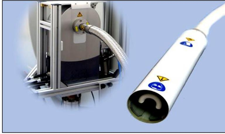
**Fig. 1.1** Bruker cryo-coil (cryoprobe) used in the thesis: radius 11mm, temp. 20K, preamplifier cooled to 77K. (<https://www.bruker.com/en/products-and-solutions/preclinical-imaging/mri/MRI-CryoProbes/rat-array-mri-cryoprobe.html>)
