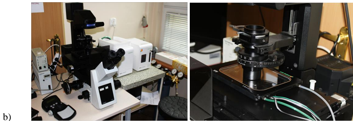
Figure 3.5. a) Scheme of the work and b) photos of the experimental device - table CO 2 incubator (Tokai Hit) mounted on the inverted optical microscope (Olympus IX83), combined with CO 2 and CO 2 /O 2 controller, allows maintaining the temperature of 37°C.
