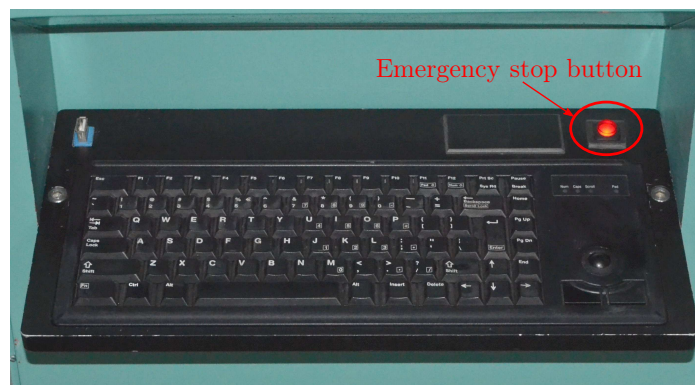
Fig. B.19: Keyboard of the large-area TL reader with emergency button marked.
