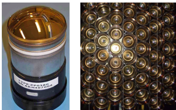
Figure 3.4: Image of a single HPD (left) and the RICH1 HPD plane (right) [62][96].
