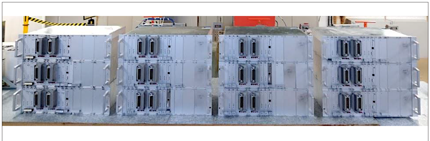
Fig. 8.6. Four sets of new AIV multiplexers. (Image copyright DAI)
