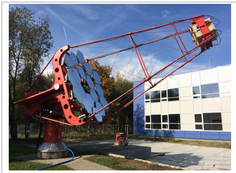
Fig. 1.22. The SST-1M imaging atmospheric Cherenkov telescope equipped with mirrors and the Cherenkov camera. The telescope is installed at the test site in IFJ PAN.
