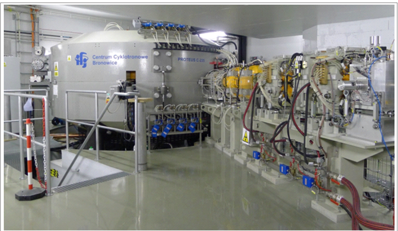
Fig. 7.1. The C 230 cyclotron – the main magnet and the beam line (quadrupoles and steering x y magnets). [Copyright K. Daniel]
