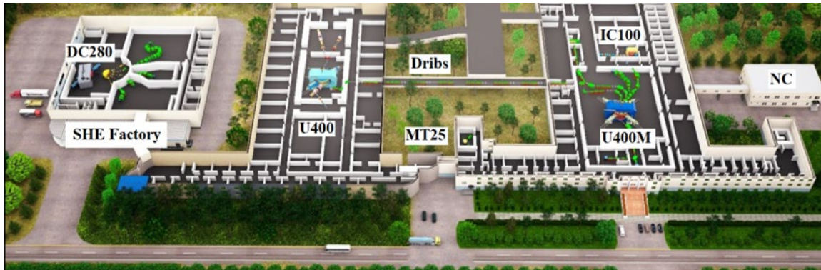
Figure 37. The layout of the Flerov Laboratory buildings. The U400, U400M, IC100, DC280 are heavy ion cyclotrons, MT25 is the microtron, SHE Factory is the Super Heavy Element Factory, NC is the Nanotechnology Centre.
