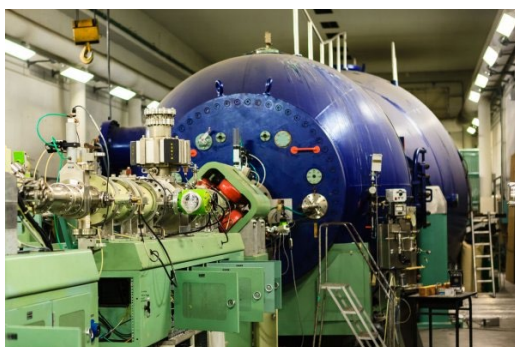
Figure 20. Pictures of the electron linac and of the Tandem accelerator (bottom) at the ALTO facility of the IJC Laboratory.
