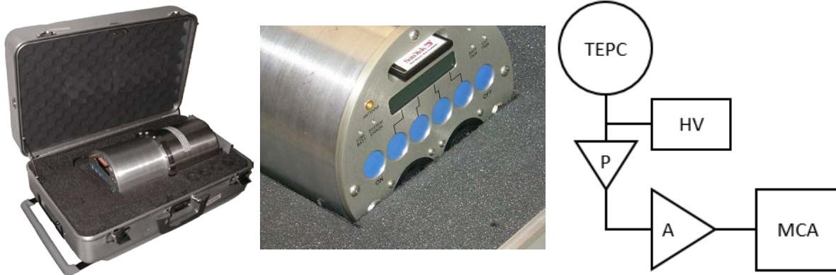
Figure 12 Hawk Environmental Radiation Monitor (left, middle). Right: typical arrangement for the measurement of the pulse height spectrum with a TEPC (HV-high voltage, p – preamplifier with CR-RC shaping circuit, A - main amplifier, MCA - multi-channel analyzer
