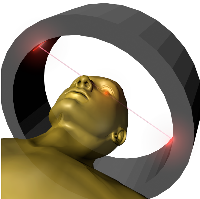
Figure 3.2. An example of emission tomography – Positron Emission Tomography. A positron emitted by radionuclide travels very short distance before it annihilates and generates the pair of gamma rays each of energy of 511 keV. The two almost back-to-back emitted photons are registered in coincidence by two external scintillation detectors in order to determine both activity and location of the positron emitter.
