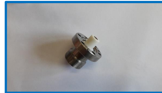
Thermal shocked Leak tight
