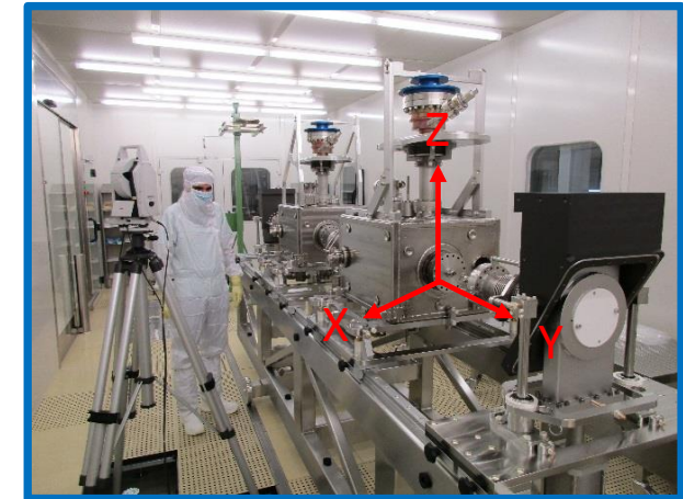
Survey done inside the cleanroom
