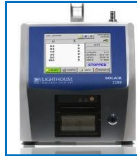
Particle counter Lighthouse 6 channels measurement From 0.3 to 10 \mu\text{m}
