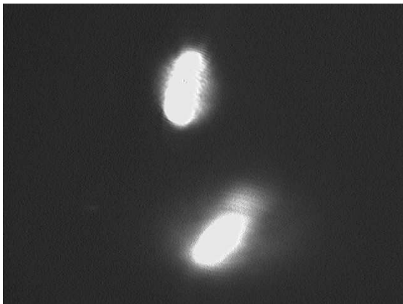
Fig. 4. The shape of two laser spots, the lower one is the 45 degree beam.
